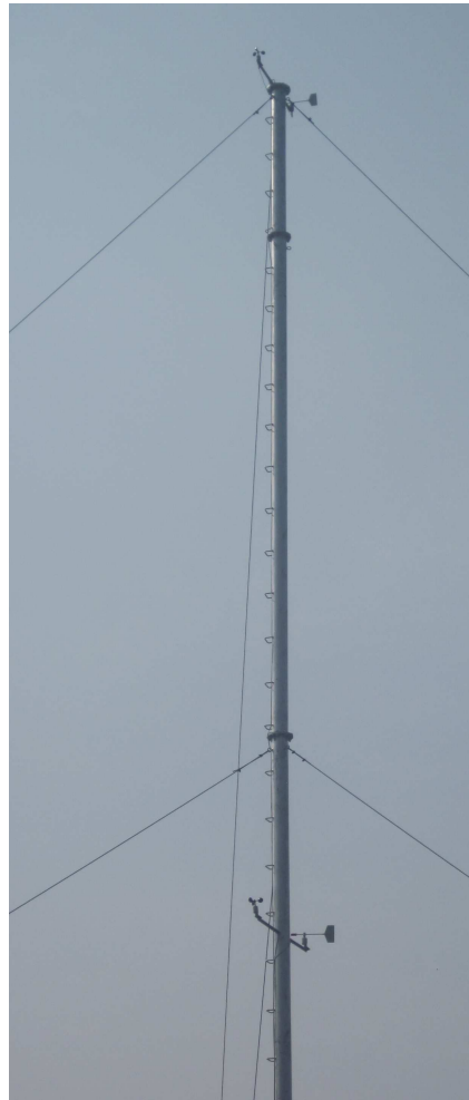
Fig. 4.5. Wind climate data measurement at 20 m (AGL) at site-I
