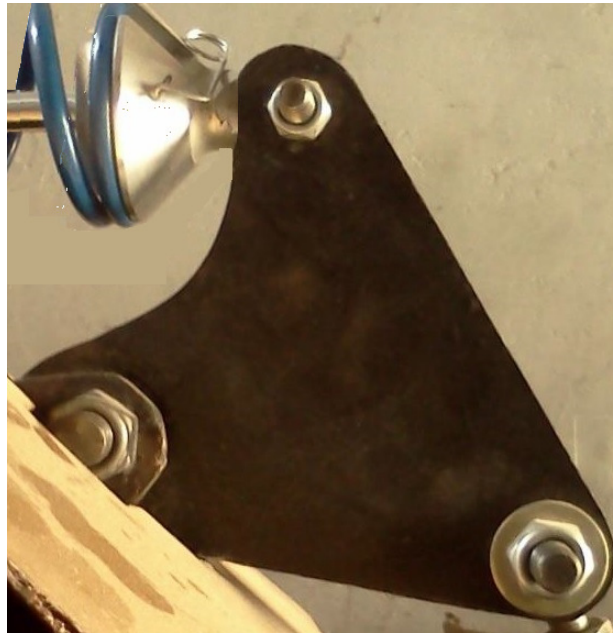
Fig. 7.6: The existing bell crank lever in the BITS Pilani formula car (Mehta 2013)
