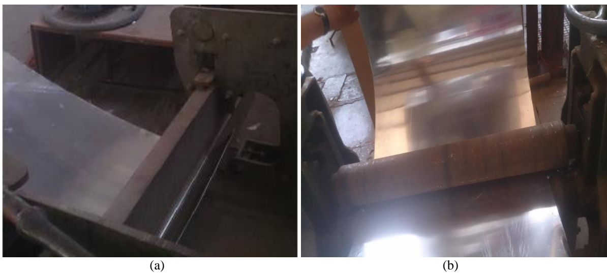
Fig. 5.3 (a) Bending of sheets at ends (b) Rolling of parabolic trough sheet
