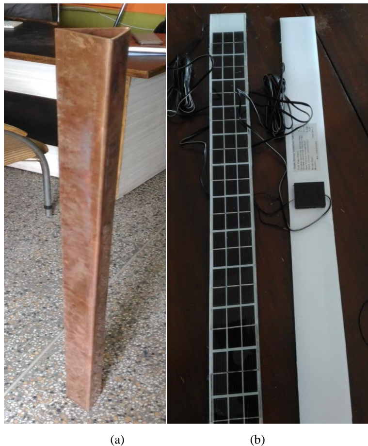
Fig. 5.9 (a) Triangular copper tube (b) PV panel to be mounted on tube
