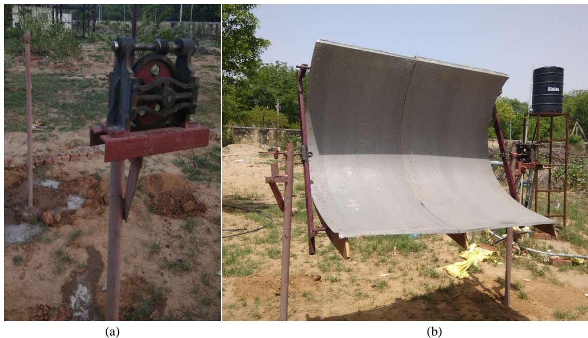
Fig. 5.6 (a) Support mechanism with worm gear based tracking mechanism (b) Final assembled parabolic trough on support structure
