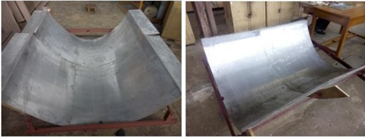
Fig. 5.5 Final parabolic trough with arms for support and screw mechanism
