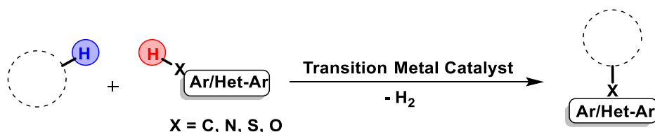
Figure 3.1 A generalized representation of the cross-dehydrogenative coupling
