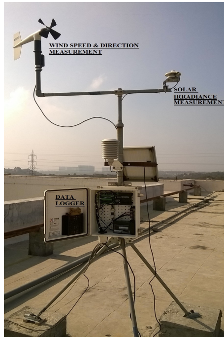
FIGURE 5.10: Weather Monitoring Systems installed at BITS-Pilani, Hyderabad
