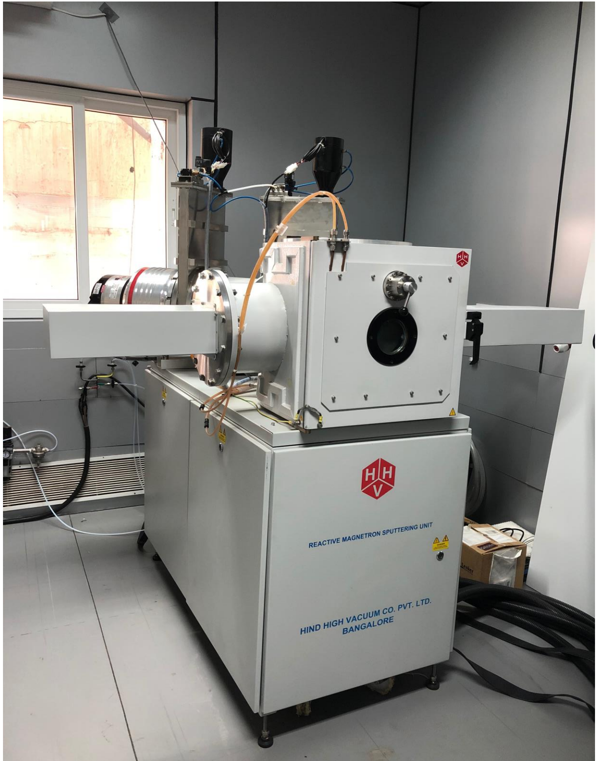
Fig. 3.8 Reactive magnetron sputtering unit in CSIR- CEERI Pilani
