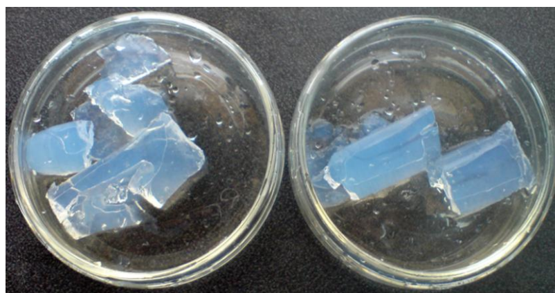
Fig. 2.1. The gel obtained after dialysis of the sol during the sol-gel synthesis of \text{TiO}_2 .
