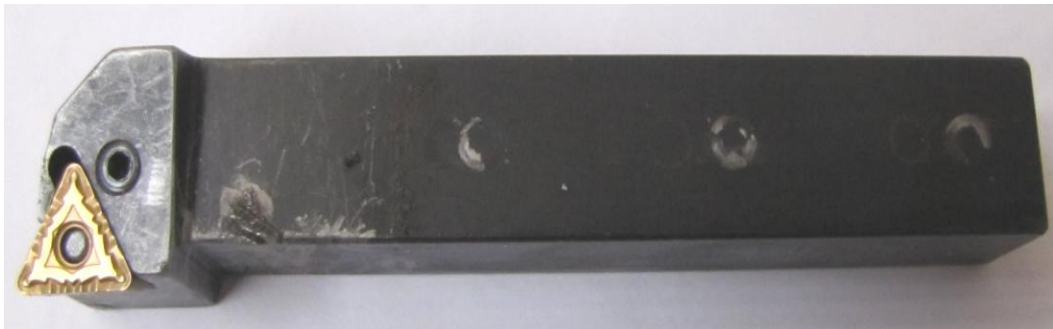
Figure 3.2: Insert mounted on the tool holder
