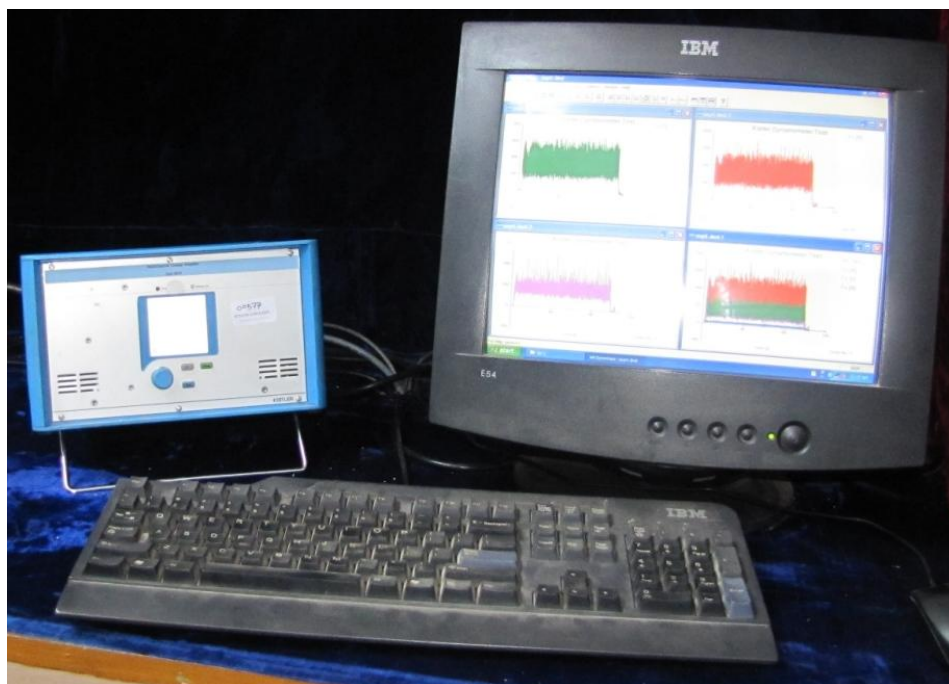
Figure 3.6: 5070A multi-channel amplifier connected to computer to process the force data
