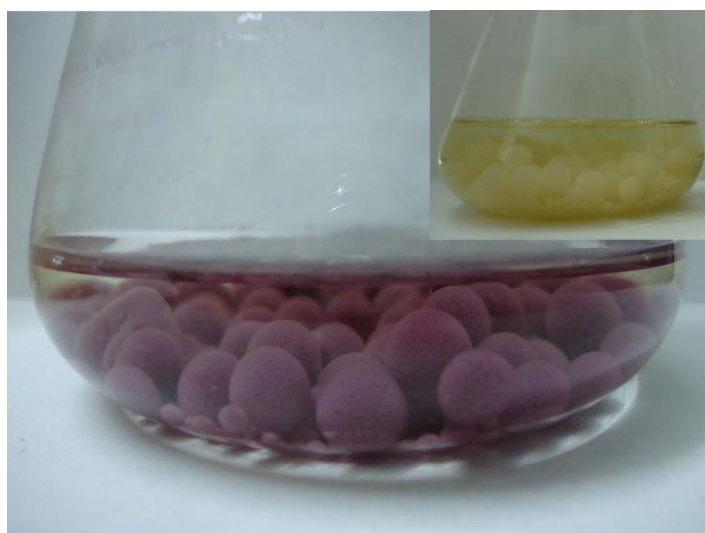
Figure 4.3 Erlenmeyer flask containing fungal biomass after 9 h exposure to gold (III) chloride (Inset shows fungal biomass before exposure)
