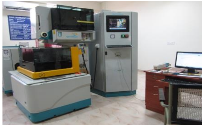
Figure (3.17) EDM used for UTM specimen.
