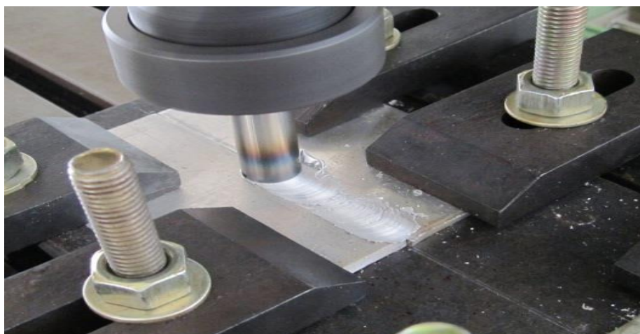
Figure (3.9) FSW process on conventional milling machine.
