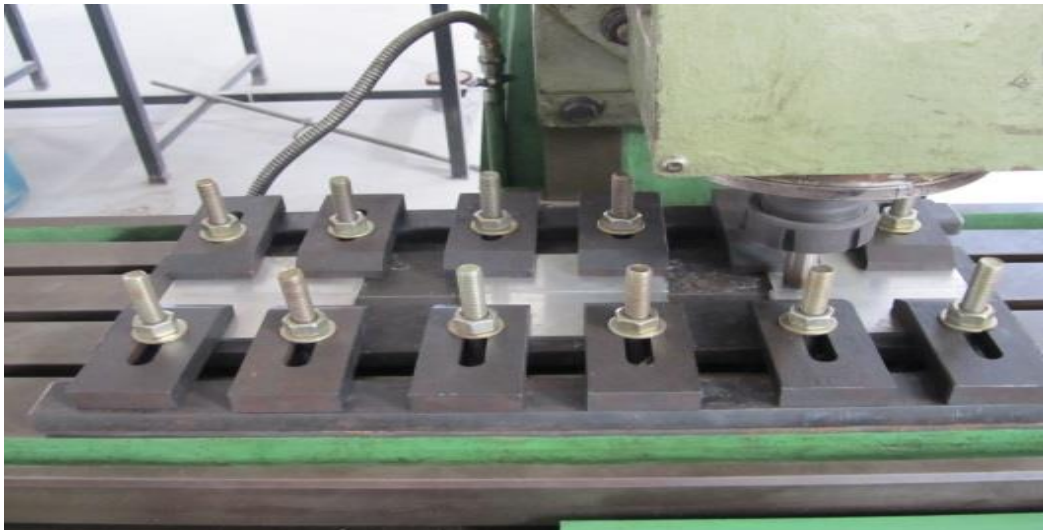
Figure (3.7) Fixture set up on the bed of Conventional milling machine.
