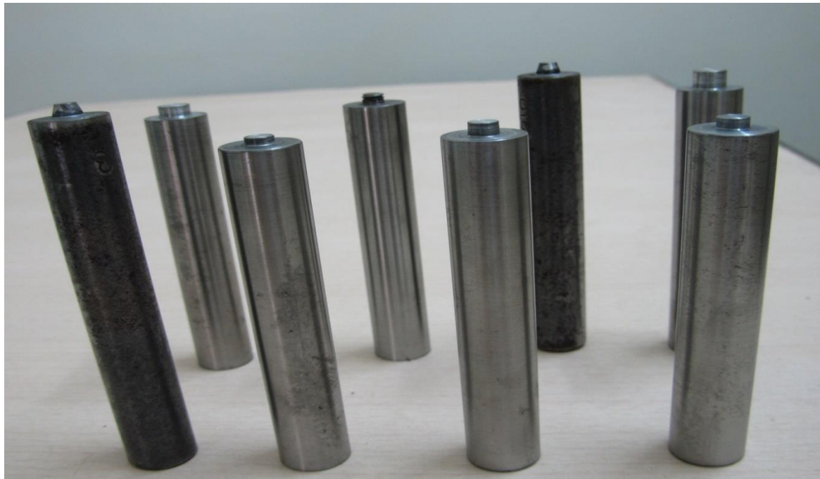
Figure (3.6) Tools used with different profiles for FSW welds.
