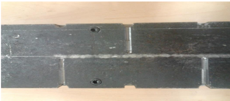
Figure (3.4) Backing plate with grooves for thermocouple seating.
