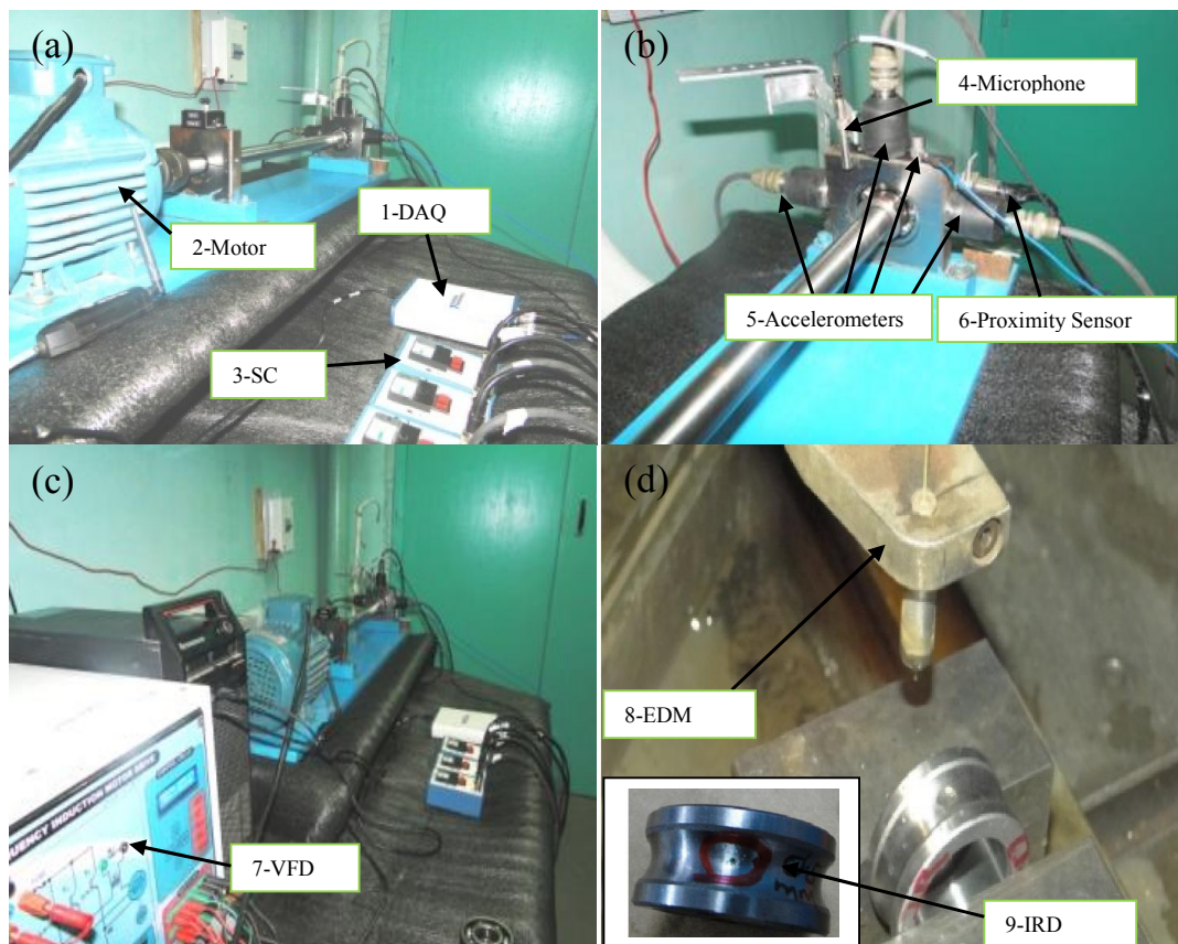
Figure 5.2 Experimental setup (a) 1-NI-USB DAQ, 2-Motor, 3-Signal conditioner (SC) (b) 4-Microphone, 5-Accelerometers, 6-Proximity sensor (c) 7-Variable frequency drive (d) 8-Electrical discharge machine, 9-IRD
