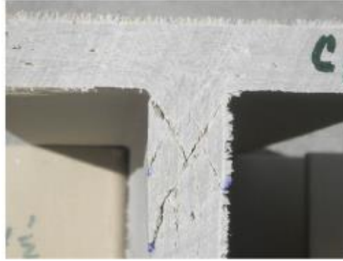
Fig. 2.2. Failure of web-flange junction (Borowicz and Bank, 2013).
