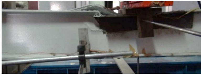
(a) Beam with carbon fiber layers (7C-CL-AS beam)
