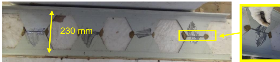
(b) Assembling of the T-sections and filling the gap with adhesive
