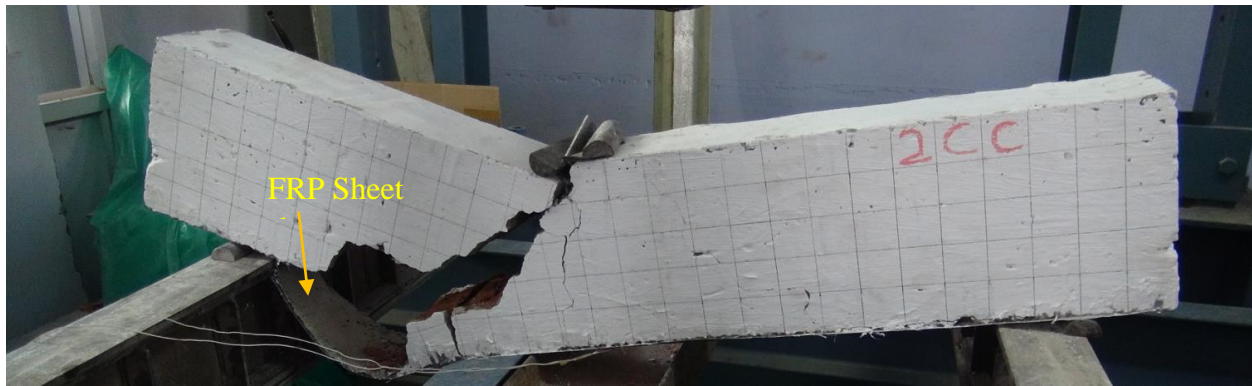
Fig. 4.14 Shear failure of Series #2 beam with cement mortar as bed joint (CM-CFB)
