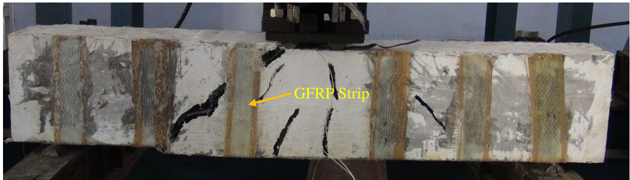
Fig. 4.18 Shear failure of Series #3 beam with ECC as bed joint (CE-GUB)
