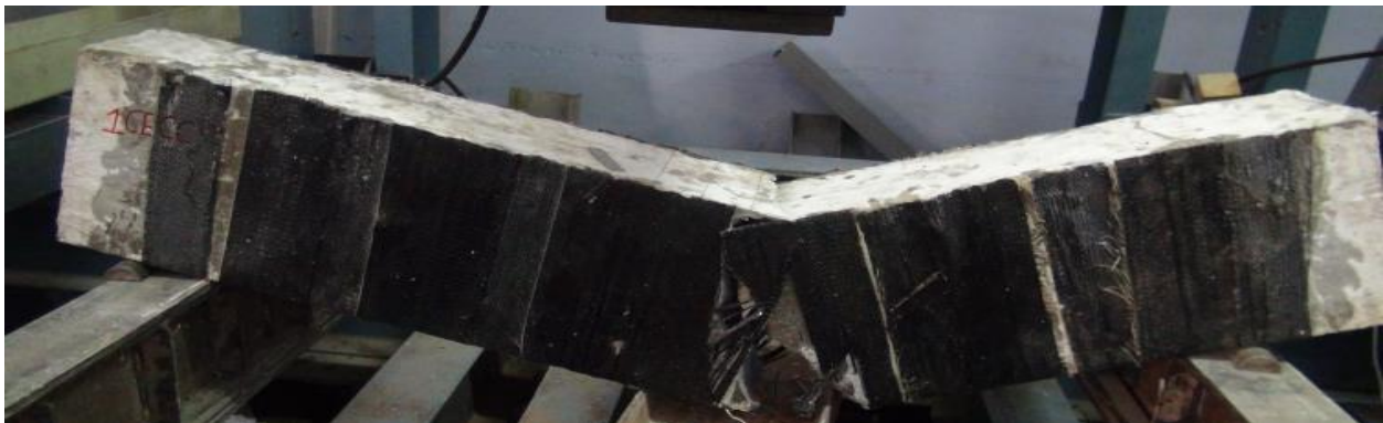
Fig. 4.21 Failure mode of Series #4 beam with ECC as bed joint (CE-CCB)
