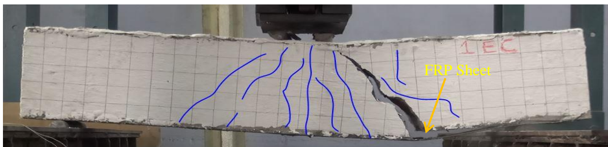
Fig. 4.15 Shear failure of Series #2 beam with ECC as bed joint (CE-CFB)
