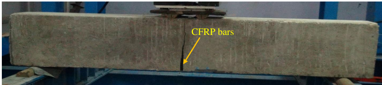
Fig. 4.24 Failure mode of reinforced beam with hand layup CFRP bars (Series #5)
