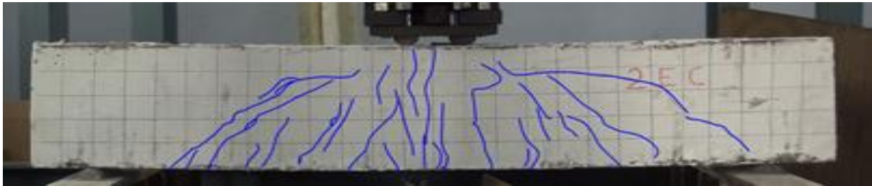
Fig. 4.12 Failure mode of control beam with ECC as bed joint (CE)
