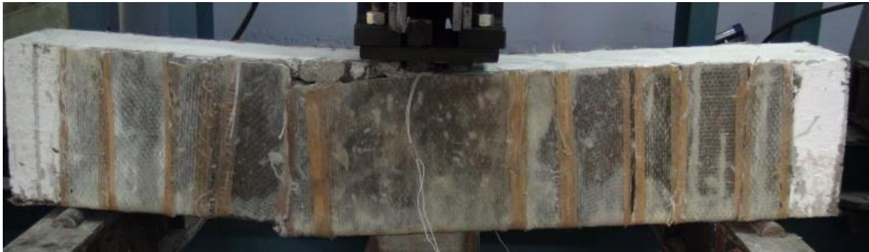
Fig. 4.20 Failure mode of Series #4 beam with cement mortar as bed joint (CM-GCB)
