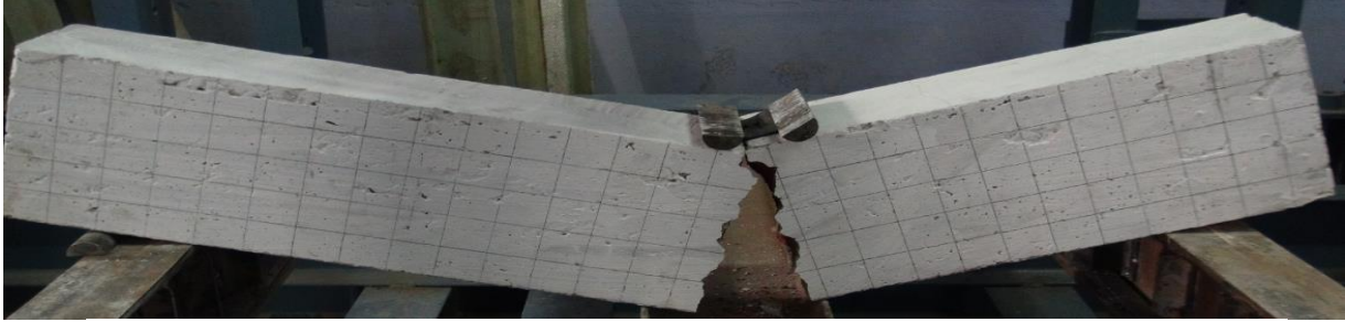
Fig. 4.11 Failure mode of control beam with cement mortar as bed joint
