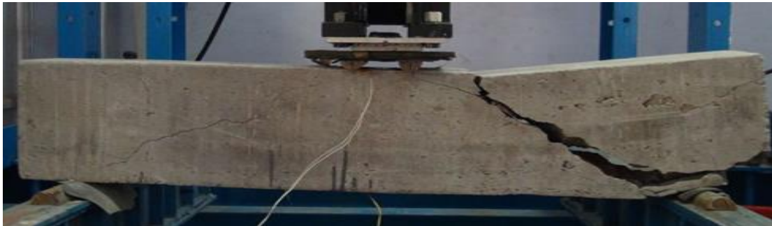
Fig. 4.26 Failure mode of NSM strengthened beam with pultruded CFRP bars
