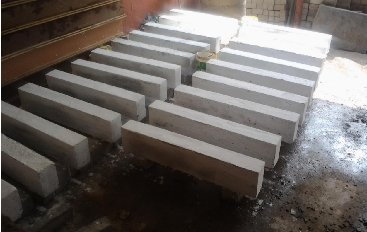
Fig. 4.1 Masonry beam specimens
