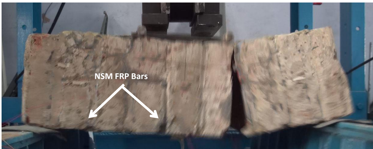
Fig. 5.14 Failure pattern of Series #3 specimen subjected to four-point loading
