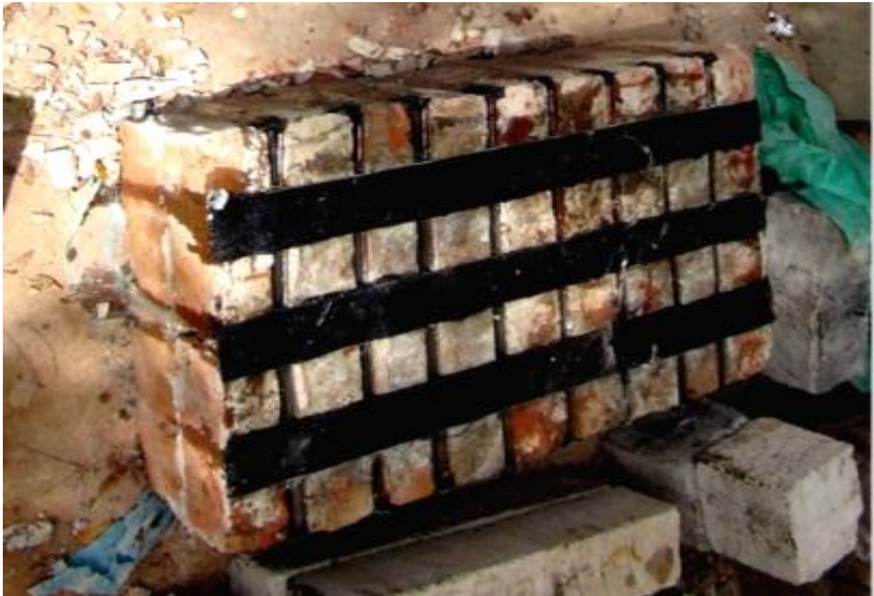
Fig. 5.5 Masonry wall with NSM CFRP bars along with CFRP strips (Series #4)
