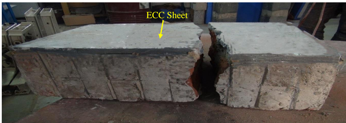
Fig. 5.17 Failure pattern of ECC strengthened masonry wall (Series #5 specimen)
