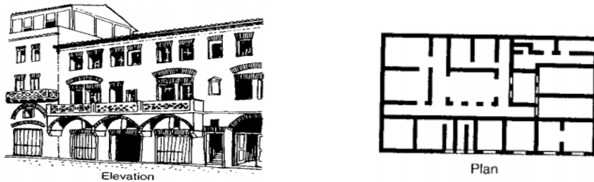
Fig. 2.1 Early multistory load-bearing masonry structure [3]
