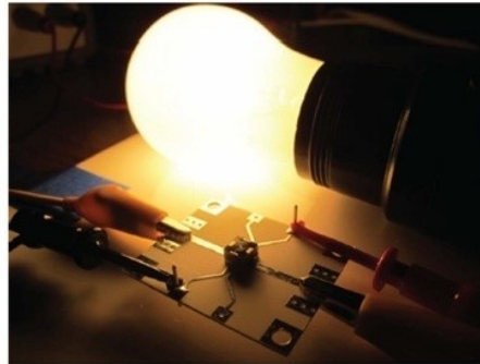
Figure 1.2: Micromechanical switch turning ON incandescent light bulb (Bachman et al., 2012)
