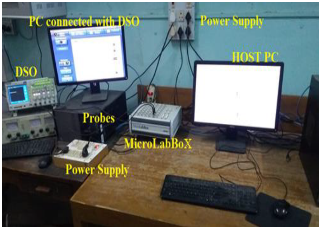
A) Hardware setup for the HIL implementation
