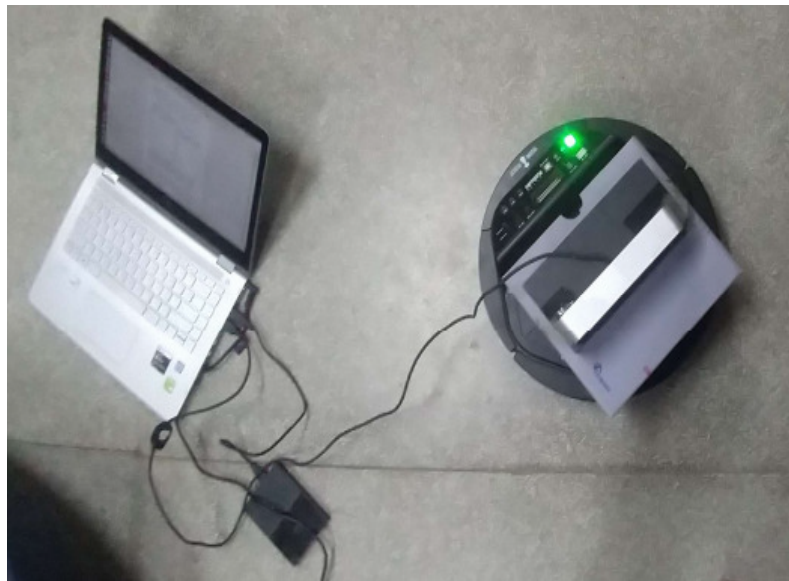
Figure 6.1: Mobile robot (KOBUKI) with vision sensor
