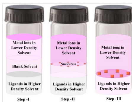
Figure 2.2: Synthesis of CPs in crystalline form through slow diffusion
