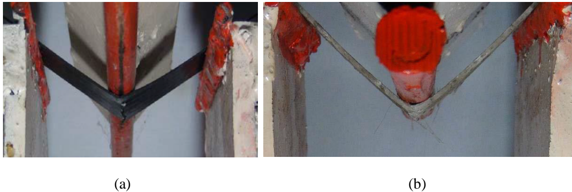
Fig. 3.33. Specimens failed after three-point bending test, (a) F-(CCCC) s (b) F-(GGGG) s
