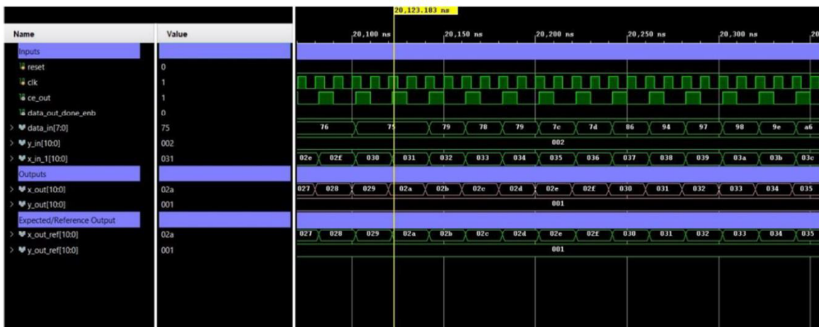
Figure 4.7. Functional RTL simulation results for HDL implementation of Sobel edge filter.
