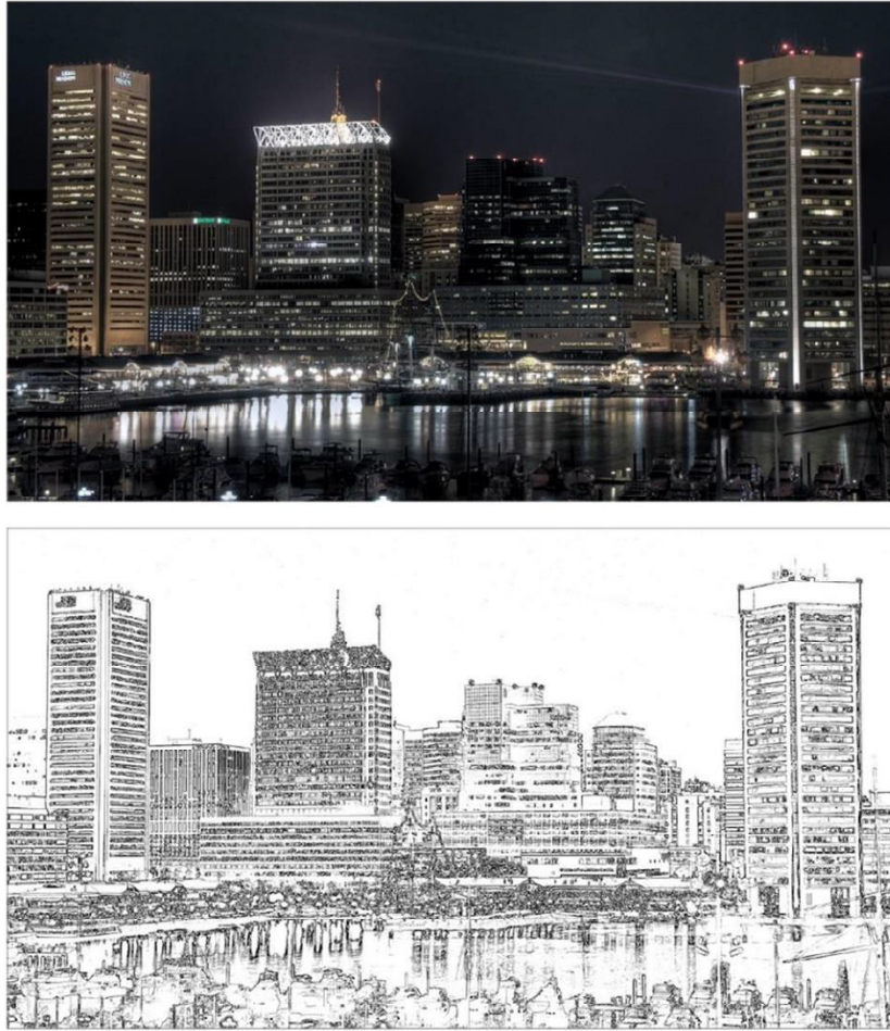
Figure 4.6. 1920 × 1080 image before and after Sobel edge filtering.
