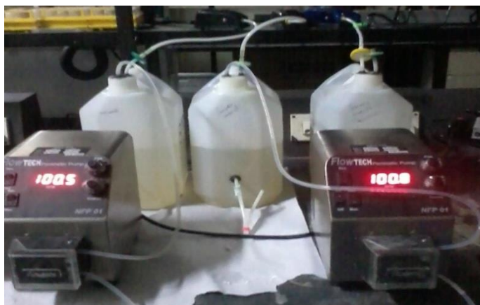
Fig 5.1: The microcosm setup for diesel degradation and HGT. The first container contains seawater, second one contains seawater + diesel, third one contains seawater + diesel + P.aeruginosa (AEBBITS 1).
