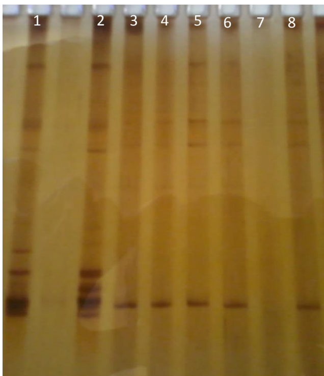
Fig 5.6: DGGE during biodegradation of diesel. First two lanes (1, 2) represent seawater on first and last day of experiment. The remaining lanes represent seawater + diesel (3, 5, 7), seawater + diesel + AEBBITS1 (4, 6, 8) on 7 th , 14 th , 21 st days respectively.
