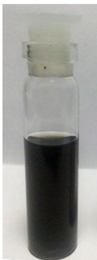
FIGURE 2.1: Solution (concentration of \sim 0.3 mg/ml) of SWCNTs uniformly dispersed in HPLC grade DMF.
