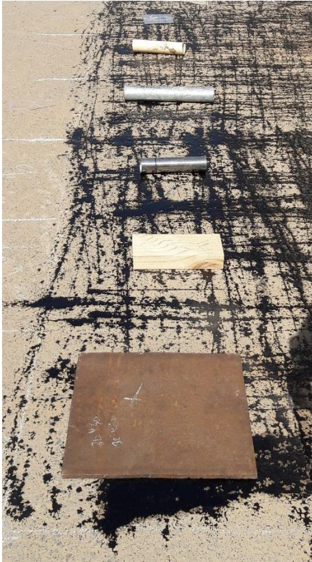
Figure 3.7. Different anomaly conditions introduced to various blocks of in-situ asphalt pavement test section
