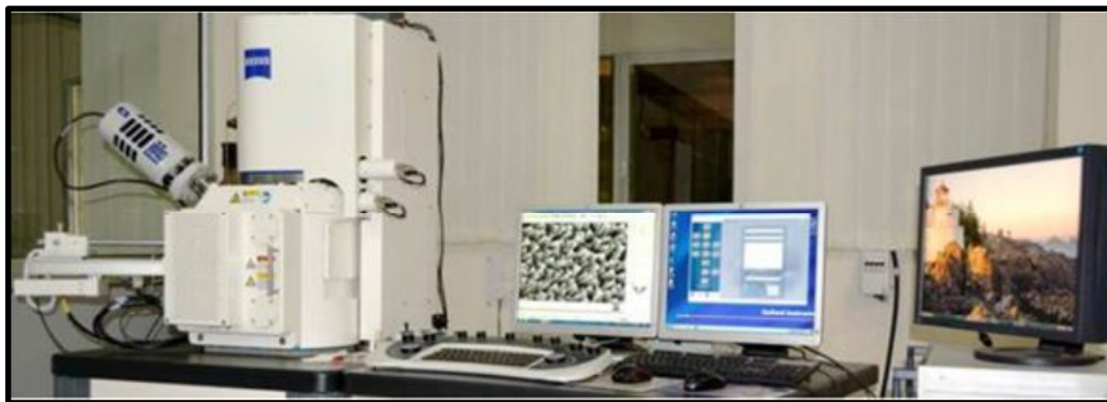
Figure 2.2: Photograph of Scanning Electron Microscope (Zeiss EVO 40).
