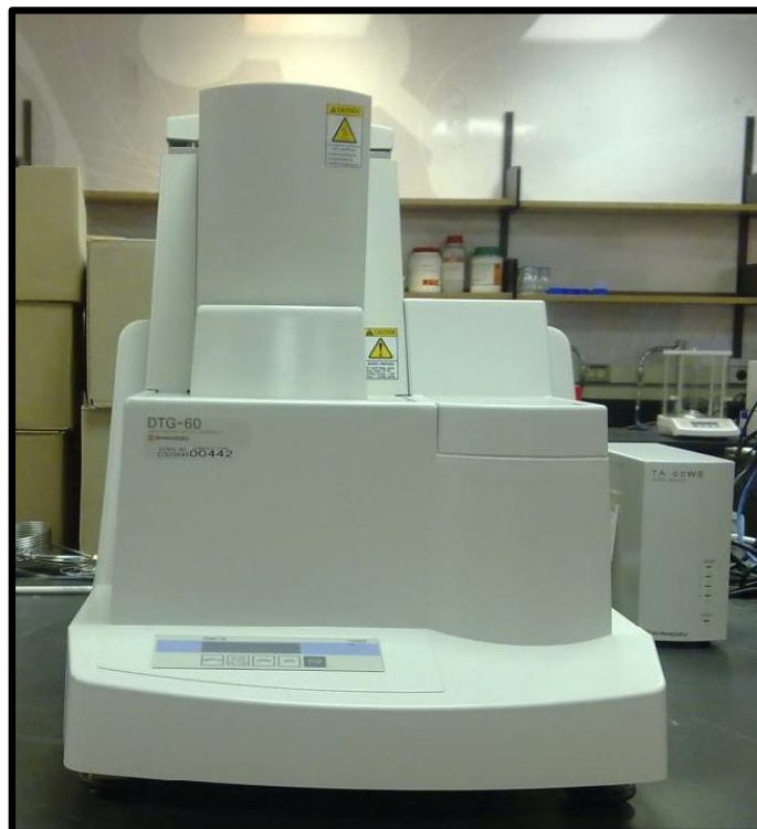
Figure 2.5: Photograph of the simultaneous thermogravimetric and differential thermal analyzer (SHIMADZU DTG-60H).
