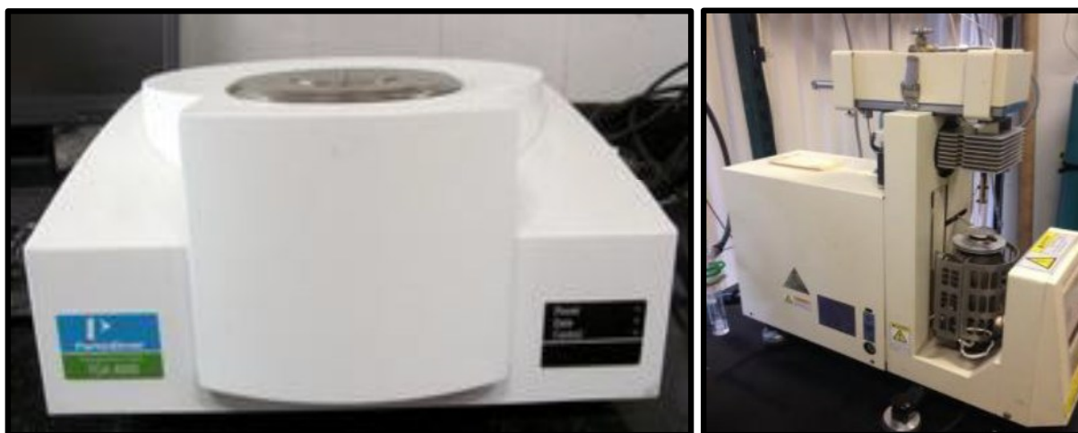
Figure 2.4: Photograph of the thermogravimetric analysis (TGA) instruments - TGA 4000 PerkinElmer and TGA-50, SHIMADZU apparatus.
