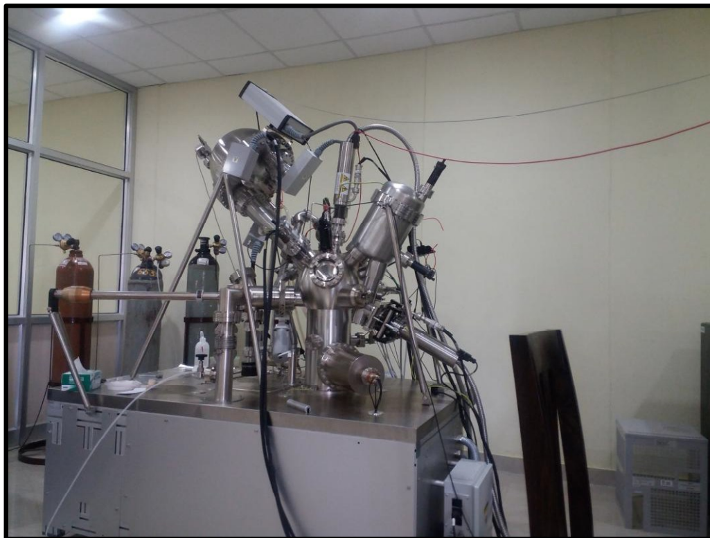
Figure 2.7: Photograph of the X-ray photoelectron spectrophotometer (Omicron EA 125).
