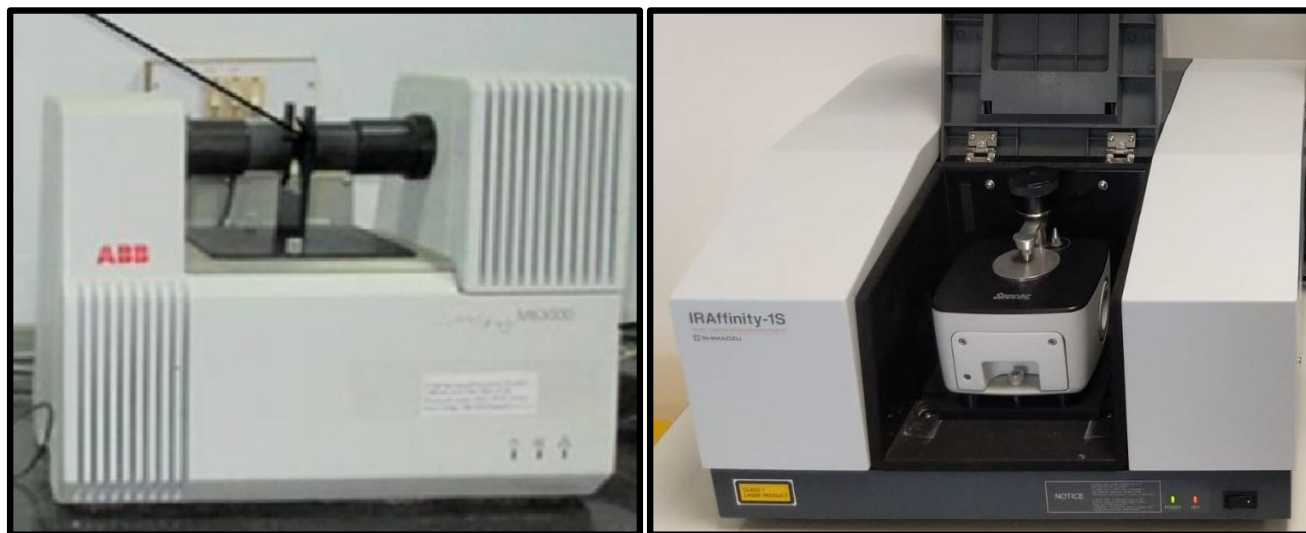
Figure 2.6. Photograph of the Fourier Transform Infrared spectrometer - ABB FTIR and SHIMADZU IRAffinity-1S.
