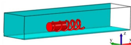
Figure 2.14: Schematic diagram of helical swimmer inside rectangular channel filled with glycerol [17]
