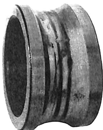
Figure 1.1 First fatigue cracks in inner raceway of a deep groove ball bearing.
