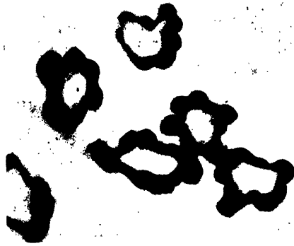
500/57 viscose rayon yarn dyed with 1 per cent. pure Benzopurpurine 4B (40 volumes) for 5 minutes at 90° C. ×400.
