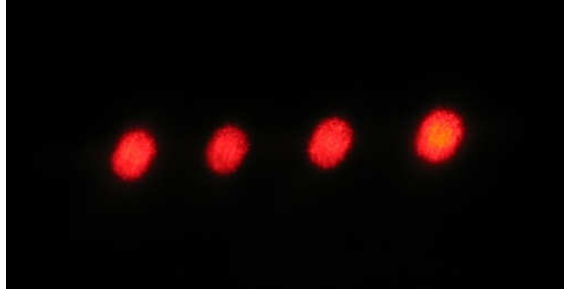
Figure 4.15. 1 \times 4 splitter output at 632.8 nm.
