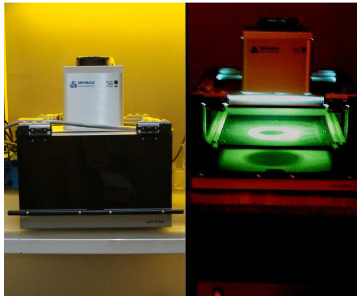
Figure 3.8. Dymax 5000 EC: Set-up (in left), during curing process (in right).
