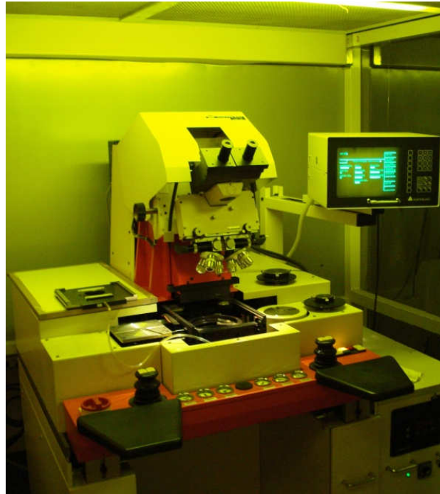
Figure 3.10. Karl Suss MA56 Mask Aligner at CSIR-CEERI, Pilani.
