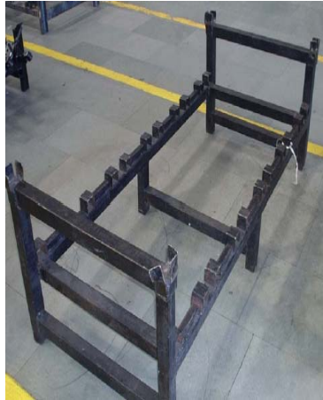
Figure 3.3a: Pallet to hold front axles (Source: Pathak, 2006)
