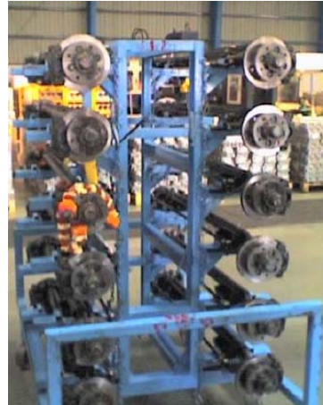
Figure 3.3b: Trolley as a standard container for holding front axles (Source: Pathak, 2006)
