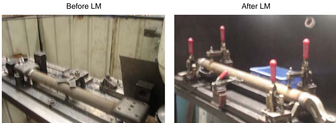
Figure 3.5: Fixture improvements carried out in the fabrication line (Source: Pathak, 2006)
