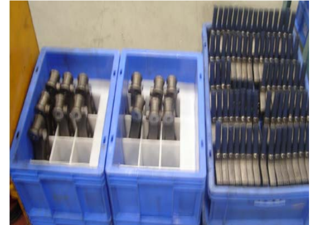
Figure 3.3c: Use of standard bins for other parts (Source: Pathak, 2006)
