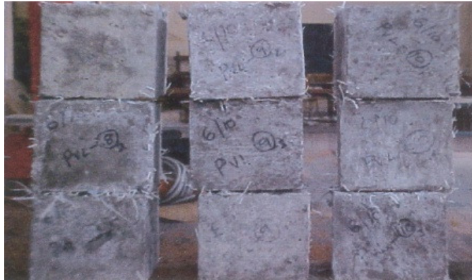
Fig.6.36 Cubes for compressive strength
