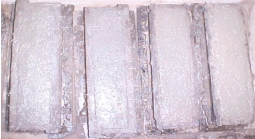
Fig.6.38 Beams for flexural strength
