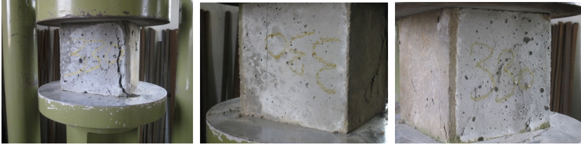
Fig. 4.4 Concrete Cubes after testing
