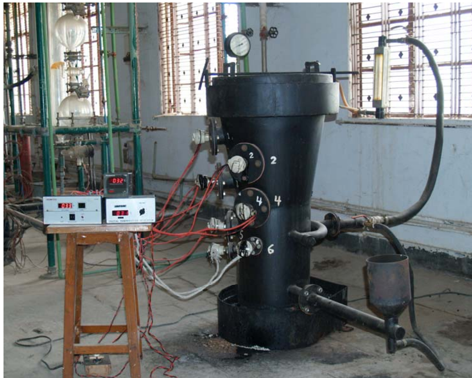
Plate-4.1 Photograph of the downdraft biomass gasifier
