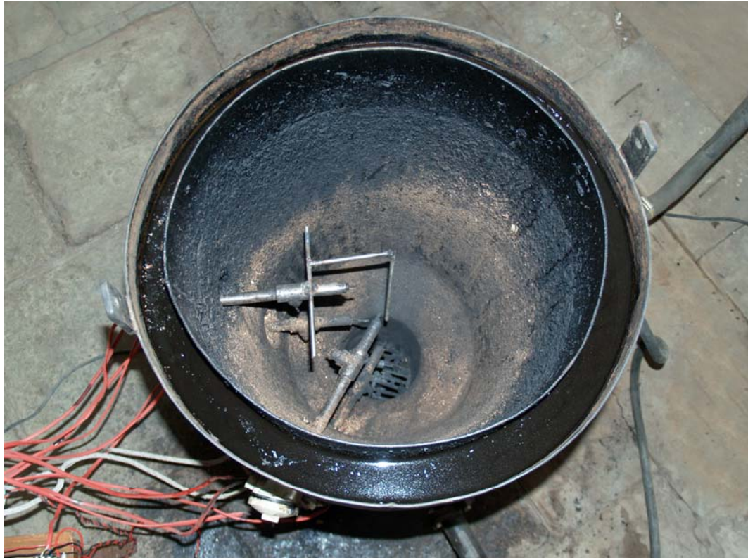
Plate 4.3 Photograph of the inside view of the biomass gasifier
