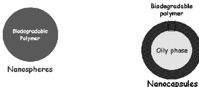
Figure 1: Schematic representation of nanosphere and nanocapsule.
