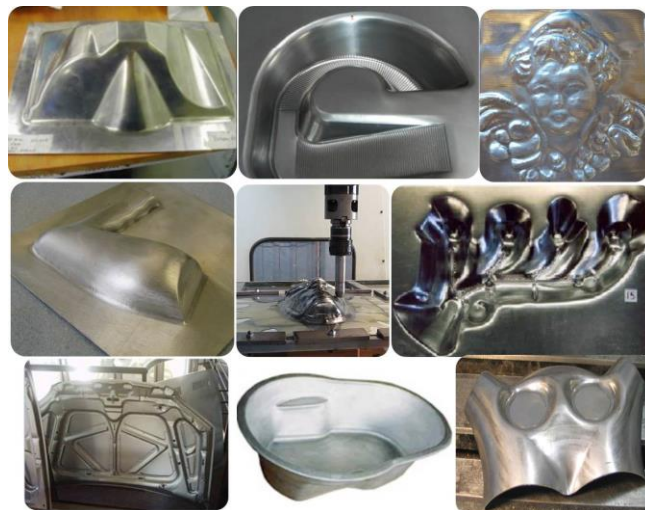
Fig. 1.5 Applications of ISF process [Jeswiet et al. (2005); Pohlak (2007); Le Van Sy (2009); Skjodt et al. (2007) www.micromanufacturing.net ]
