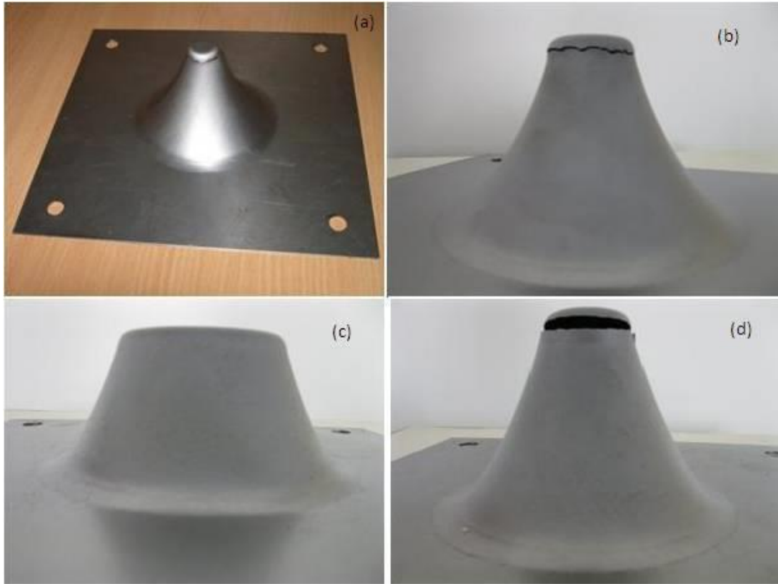
Fig. 4.4 Varying wall angle conical frustums formed in ISF
