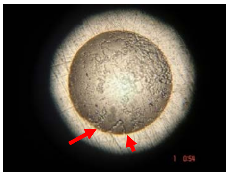
Fig 6. 7 Photograph of indentation observed under microscope for the material ST 17-4PH
