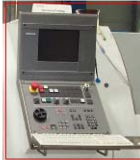
Fig 3. 11 Control panel of GILDMEISTER CTX 400 Serie2 lathe
