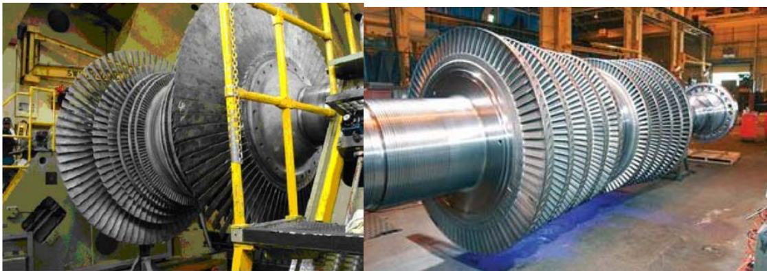
Fig 1. 1 Typical HP and LP turbine rotor (James et al, 2010)
