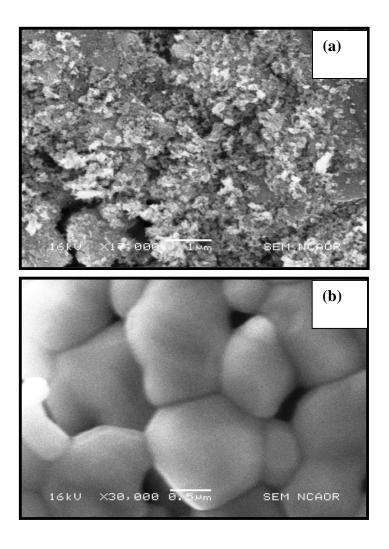
Fig. 3.4 SEM micrographs of  $\alpha$ -Fe<sub>2</sub>O<sub>3</sub> powder (a) calcined at 450<sup>o</sup>C (b) sintered at 1100<sup>o</sup>C.
