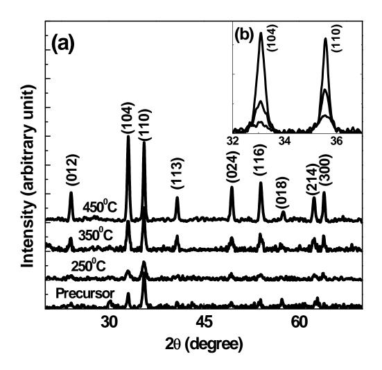
Fig 3.2 (a) X-ray diffraction spectra of precursor powders at different calcination temperatures (b) slow scan of the (104) and (110) diffraction planes.
