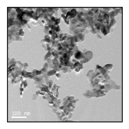
Fig 3.3 TEM micrograph of  $\alpha$ -Fe<sub>2</sub>O<sub>3</sub> powder calcined at 450<sup>o</sup>C.
