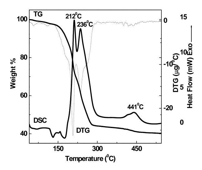
Fig.3.1 TG-DTG and DSC thermograms of the precursor in air.
