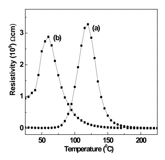
Fig. 3.5 Variation of DC resistivity with change in temperature of  $\alpha$ -Fe<sub>2</sub>O<sub>3</sub> powder for (a) unsintered sample (b) sample sintered at  $1100^{0}$ C.
