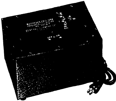
FIG. 175.— Audio-frequency oscillator. When the cord is connected to a 110-volt 60-cycle lighting circuit, a small amount of 1,000-cycle current is available at the binding posts on the top of the case. This is a sufficient source for one of the bridges described in the following chapters. (Courtesy of the Central Scientific Co.)
