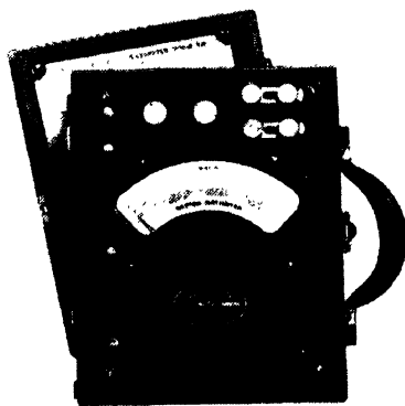
FIG. 250.—An electrodynamicometer wattmeter. (Courtesy of the Weston Electrical Instrument Co.)
