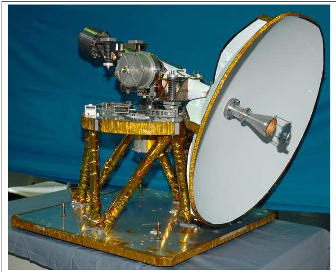
Fig. 6.2 : Dual gimbal controlled paraboloid antenna
