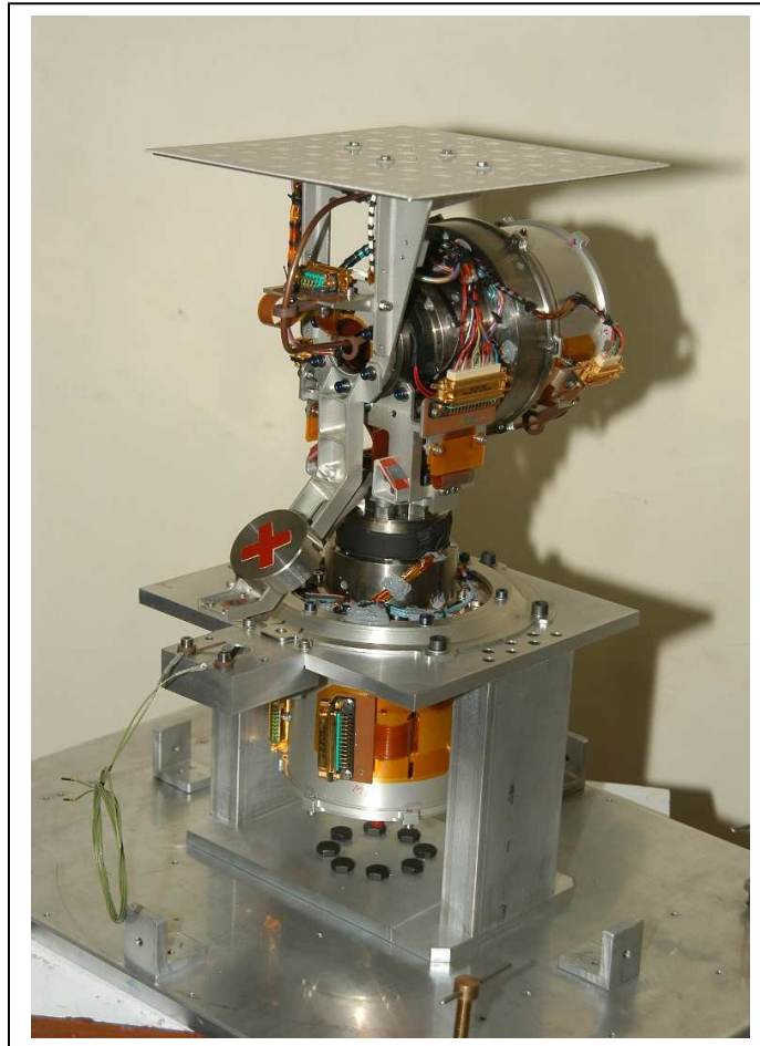
Fig. 6.3 Dual gimbal mounted planar phased array antenna of Cartosat-2
