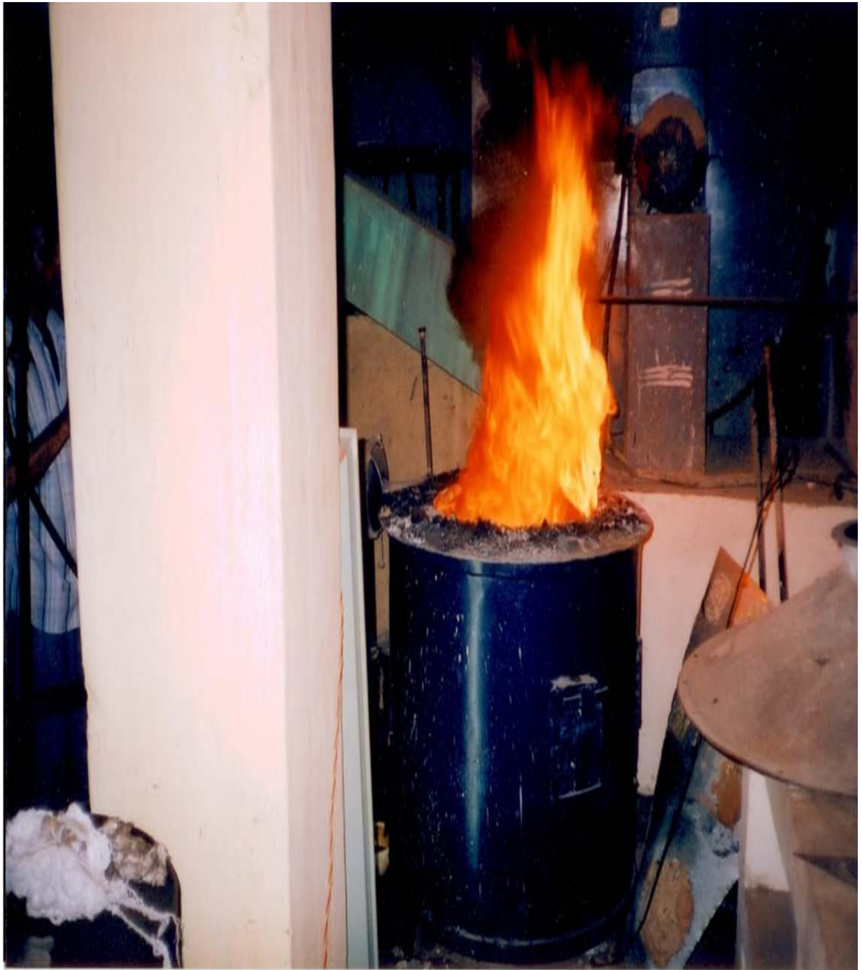
Plate.5 Combustion of Biomass slurry for 20% excess air-Top open furnace
