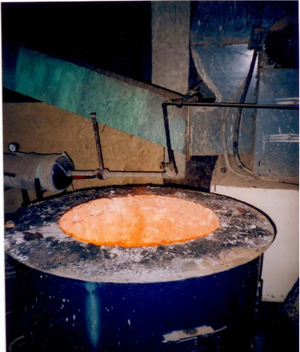
Plate.4 Combustion of Biomass slurry at stoichiometric air flow- vertical position – Top open furnace
