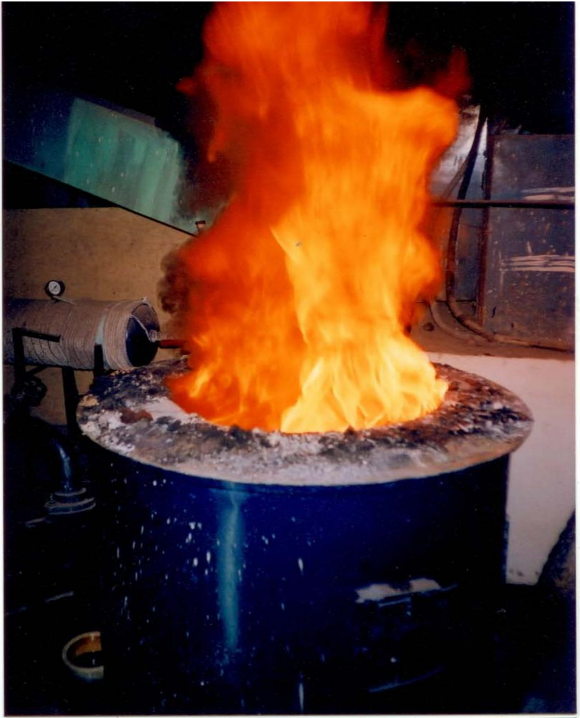
Plate.6 Combustion of Biomass slurry for 30% excess air flow-Top open furnace
