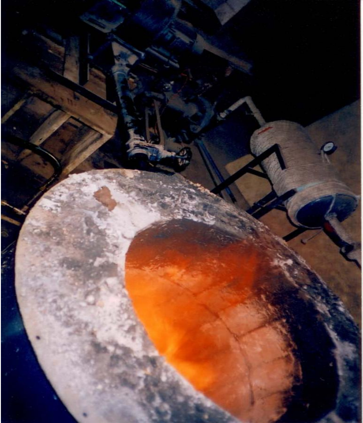
Plate.3 Combustion of Biomass slurry at stoichiometric air flow – photo taken at an oblique angle- Top open furnace
