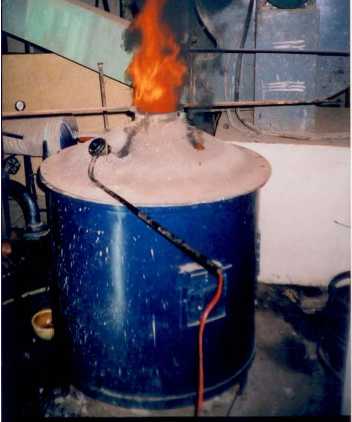
Plate.7 Combustion of Biomass slurry with top partially closed for 20% excess air
