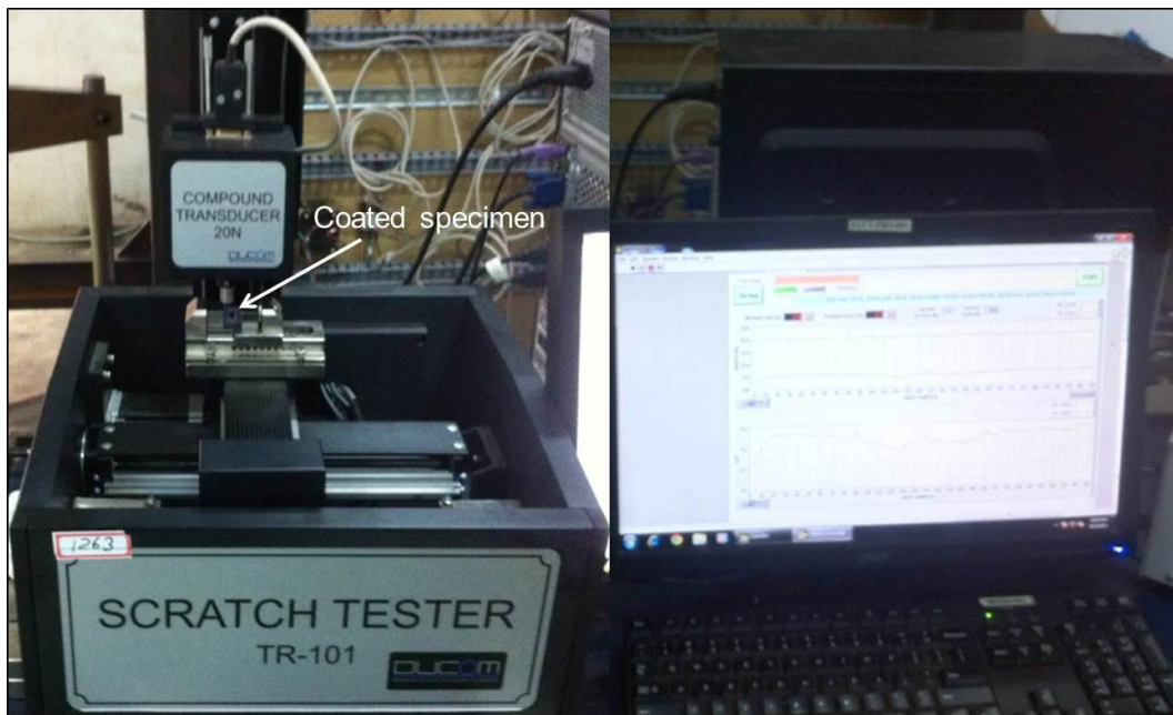
Fig. 4.5. Coating strength test using standard scratch tester (Ducom Instruments).
