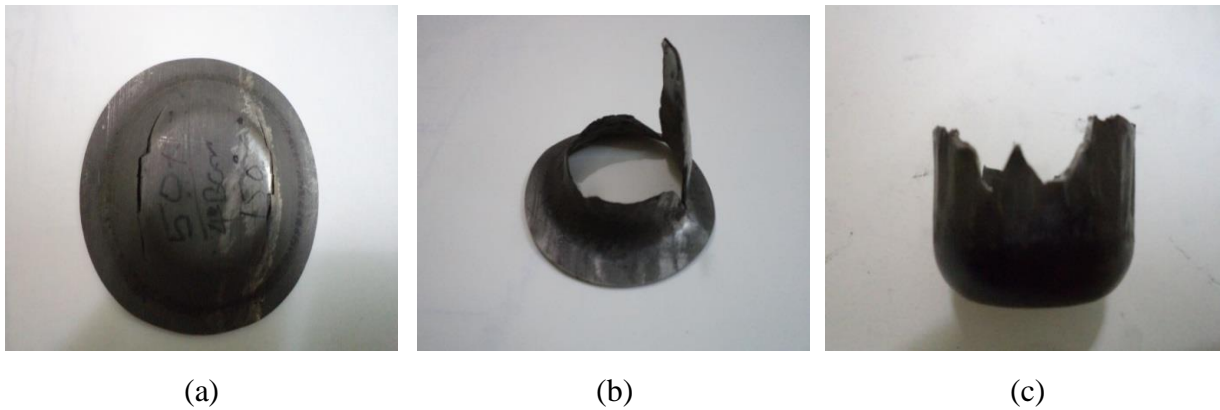
Fig.3.16: Type of failures occurred during experimentation (a) neck failure at 50 0 C (b) neck failure at 100 0 C (c) fracture at upper wall at 400 0 C
