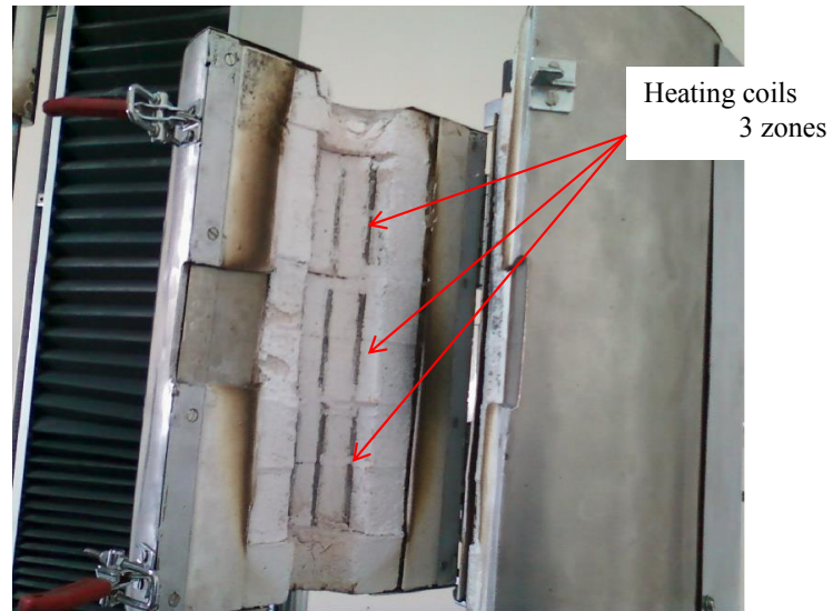
Fig.3.3: 3-zone split furnace attached to UTM for high temperature tensile testing
