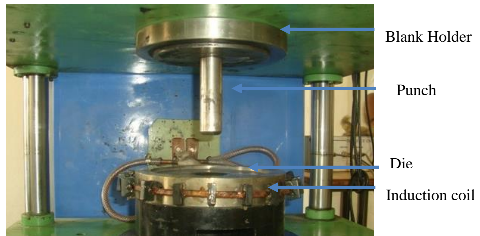
Fig. 3.14: Induction heating coil arrangement for deep drawing process up to 400 0 C
