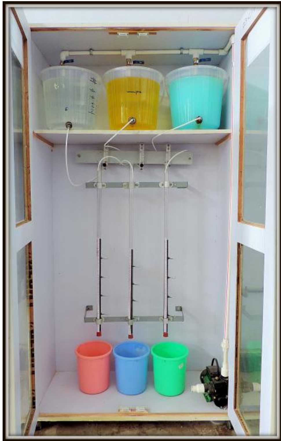
Plate 3.3: Photograph of experimental setup for continuous adsorption process.
