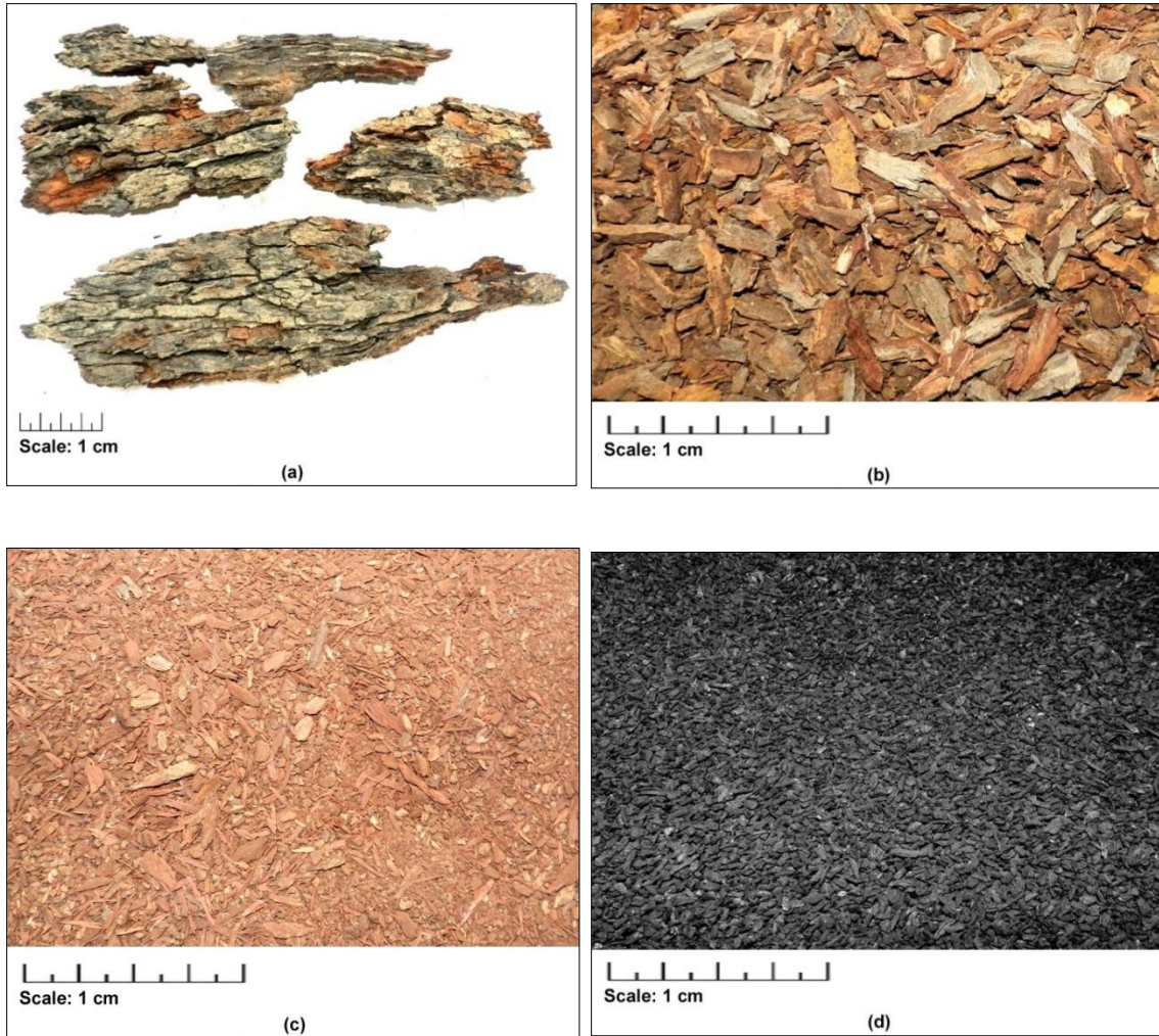
Plate 3.1: Photograph of (a) Fresh Neem Bark; (b) Neem bark after first crusher; (c) Neem bark after final crusher; (d) Neembark after activation; the different stages of preparation.
