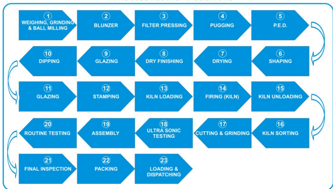
Figure 5.5: Production process for the insulators
