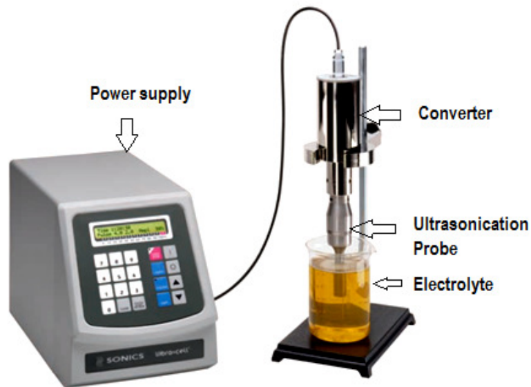
Figure 3.13: Image of ultrasonication equipment used for the ultrasonication Model: Sonics vibra cell VC 505 (20 kHz and 500 W )
