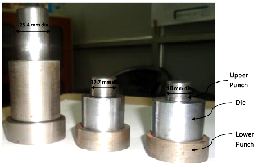
Figure 3.17: Dies used for the fabrication of the pellets
