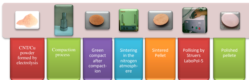
Figure 3.18: Description of pellet forming by powder metallurgy method
