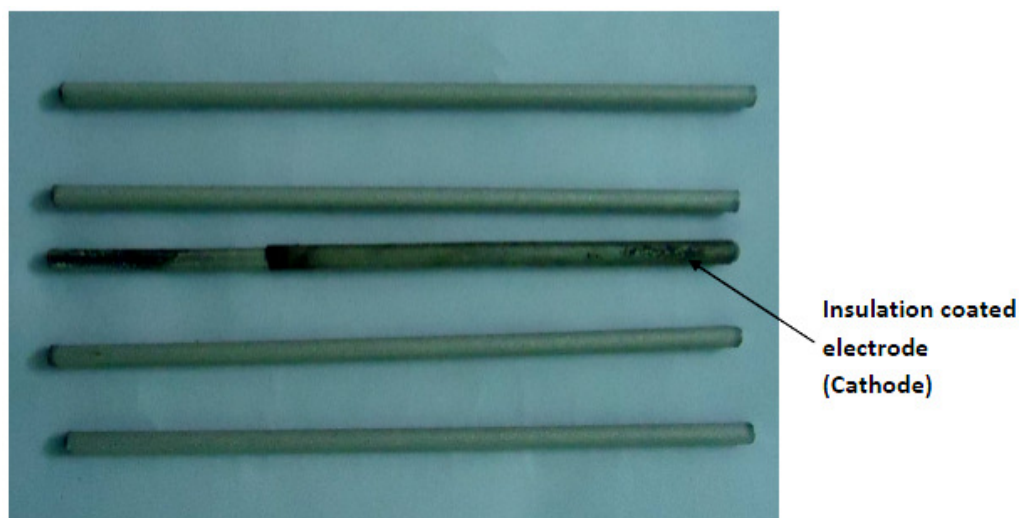
Figure 3.10: Image of titanium electrodes coated with platinum (four anodes and a insulation coated cathode)
