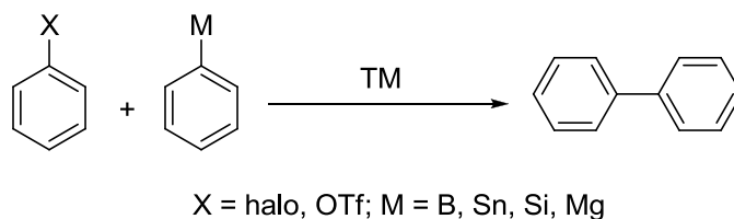
Scheme 4.1 General representation of traditional cross coupling reaction
