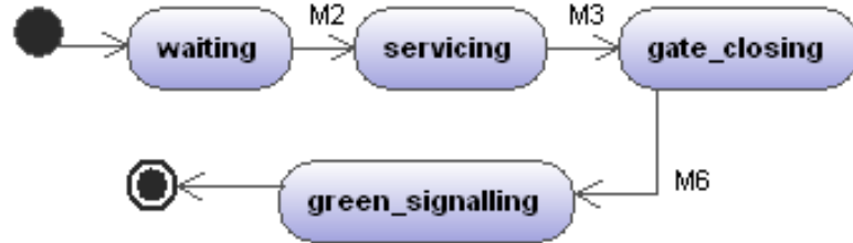
(a) CrossController State Diagram for Normal Scenario
