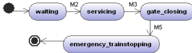
(b) CrossController State Diagram for Emergency Scenario
