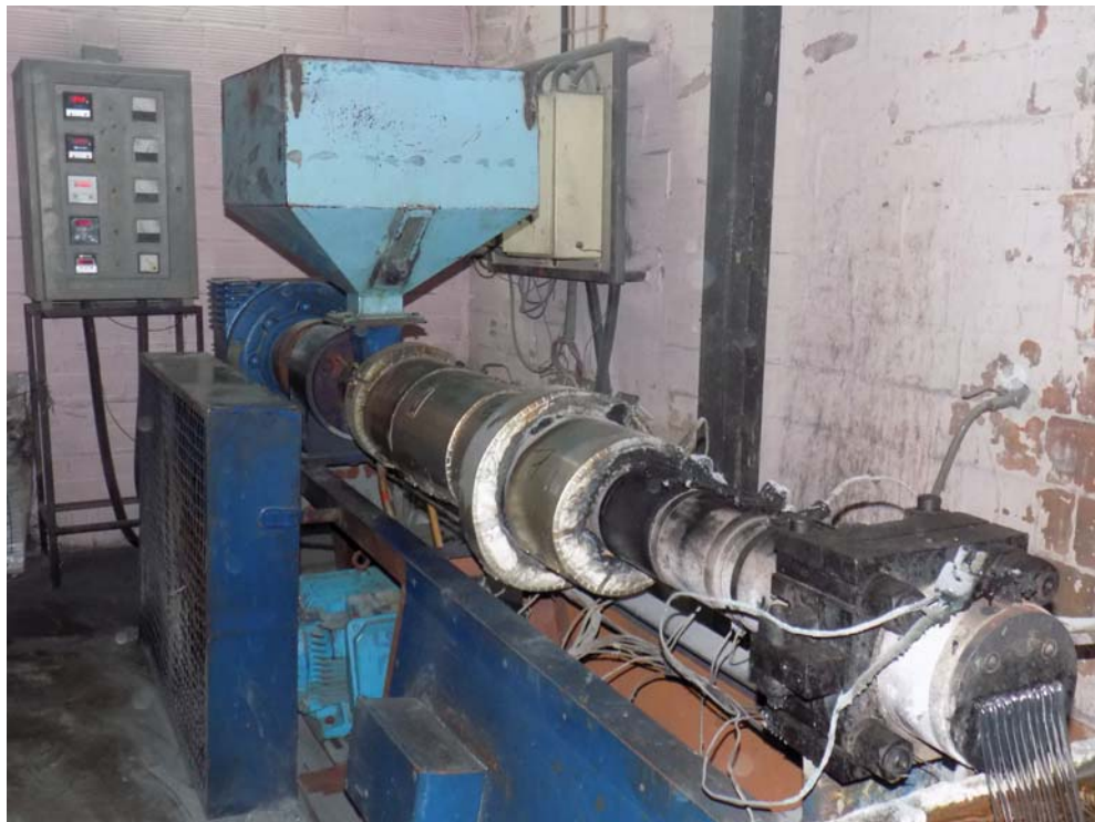
Figure 7.1: Industrial melt extruder (Courtesy: Kenwood Industries).
