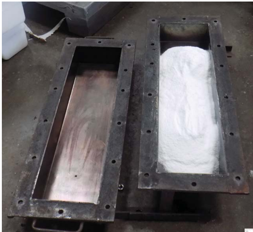
Figure 7.3: Mold used for rotational Molding - Baffle (Courtesy: GMI Zarahak Moulders) scale bar 1" shown.
