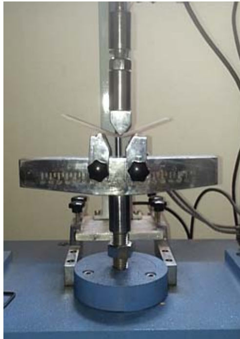
Figure 5.2: Experimental set up - flexural testing
