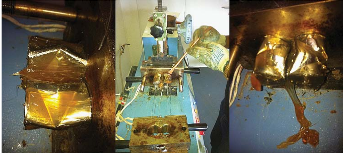
Figure 3.21: Degraded LLDPE - 8% FS blend during torque rheometry at 210°C
