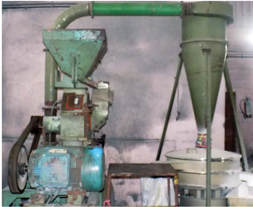
Figure 7.2: Industrial pulverizer and vibro-screen (Courtesy: Kenwood Industries).
