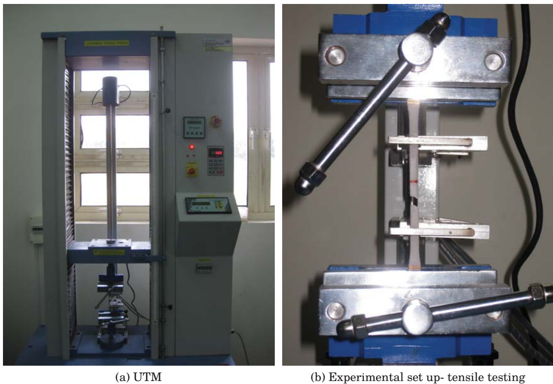
Figure 5.1: Universal testing machine and experimental setup for tensile testing
