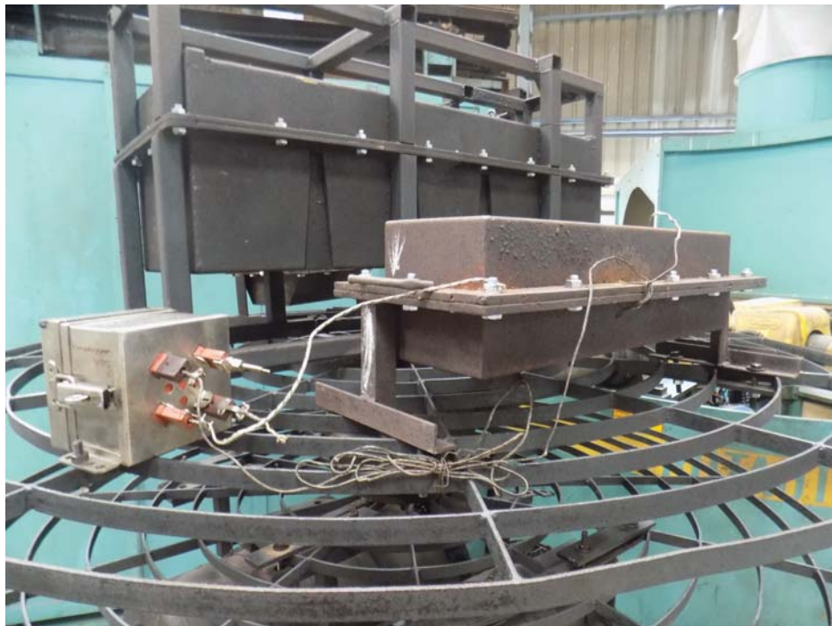
Figure 7.5: Experimental set up for IAT measurements using TEMPLOGGER™ (Courtesy: GMI Zarahak Moulders).
