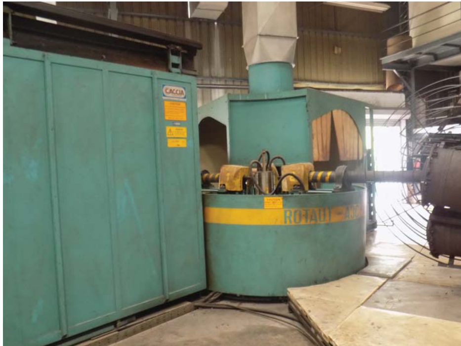
Figure 7.4: Rotational molding machine-CACCIA-RT 2203B (Courtesy: GMI Zarahak Moulders).
