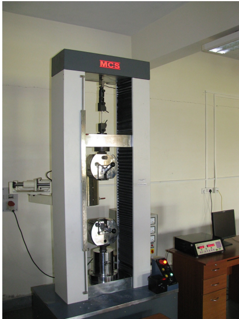
Fig. 3.7 Universal Testing Machine set-up
