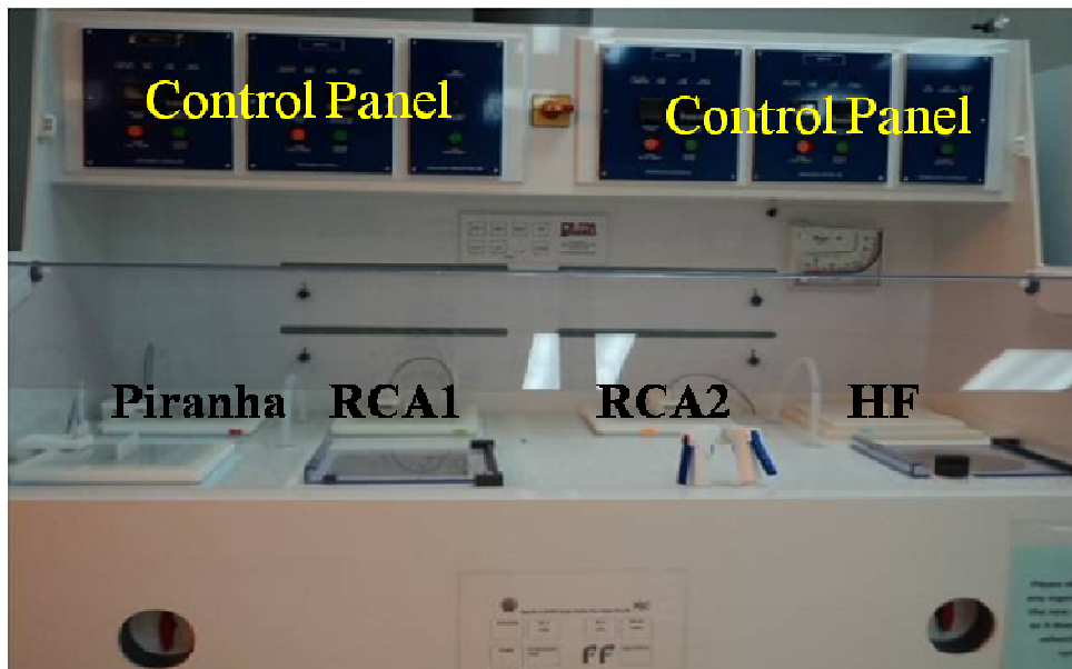
Figure A-1: Chemical wet bench setup for cleaning and etching purpose
