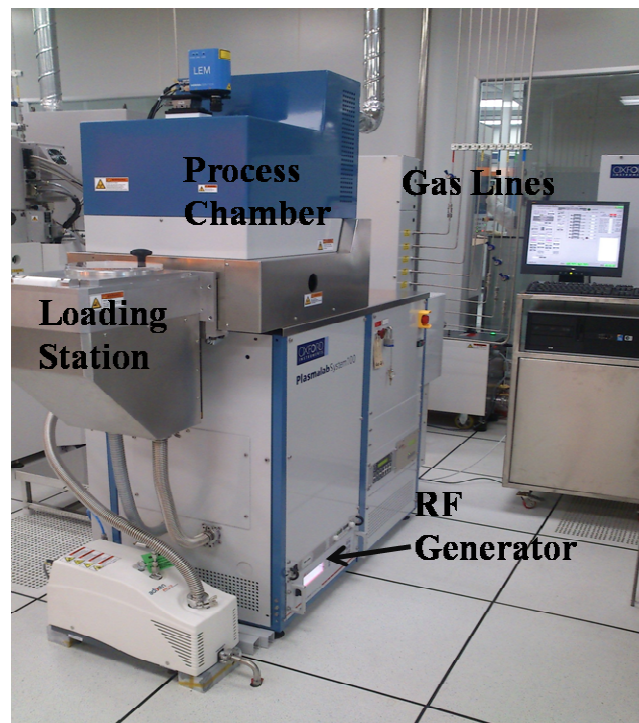
Figure A-2: Reactive ion etching system
