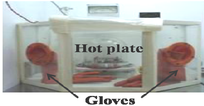
Figure A-3 Glove box for silanization
